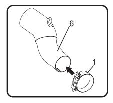
Install (No. 2) 03019143, exhaust clamp to (No.7) 11211-427, right tail pipe. **Do not torque at this time.**
