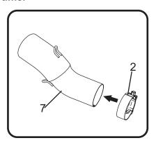
2. Install (No. 9) *HT SHLDR77*, muffler clamp heat shields to (No. 5) *1121-MPCR(X)*, muffler clamps and slide onto both mufflers.
