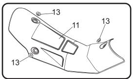
Align and install (No. 11) *12401-CFHS*, heatshield onto the two heatshield brackets on the muffler and stock header heatshield bracket using (No. 12) *RC116HSB-BK-P*, 6mm heatshield screws and (No. 14) *93412A423*, rubber dampening washers as shown on the assembly diagram.
