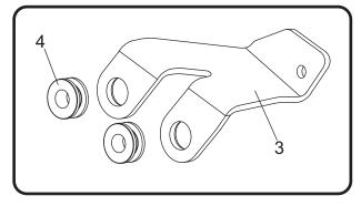
Install (No. 3) 12401-BRKT, muffler mount bracket onto stock muffler chassis mount using (No. 9,10) M8X25 and 8MMWASHER, 8mm bolt and washer.
