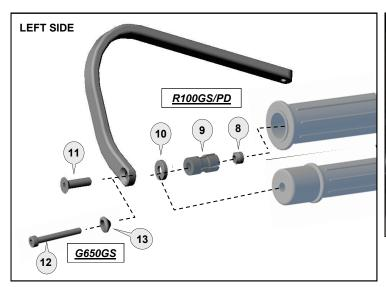
Loosely assemble clamp to the handlebar with applicable parts. Attach the handguard backbone with applicable parts to the handlebar end and also to the clamp connector (7).
