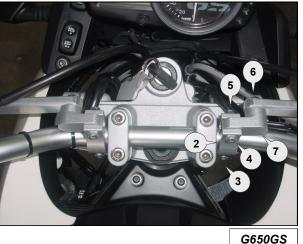
Important: Be sure to tighten clamp bolt (4) before bolt (3) to securely lock the clamp connector (7) between the two clamp halves (2).
