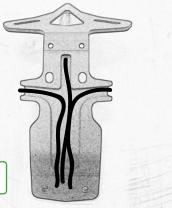
Run wires neatly down the channel in both parts ensuring they do not get trapped or squashed
