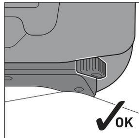
**Step [1]:** Place the four locking openings of the side case (1) onto the guide bolts of the mounted SW-MOTECH side carrier.
