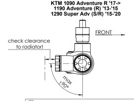
$\overline{\langle * \rangle}$  torques A: 5-9Nm / 44-80Lbs.ln / 4.0-6.4Lbs.Ft B: 14-17Nm / 124-150Lbs.ln / 10.3-12.5Lbs.Ft C: 6Nm / 53Lbs.ln / 4.4Lbs.Ft
