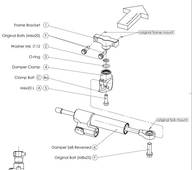
\* TORQUES [use Loctite 243 or similar] A: 5-9Nm / 44-80Lbs.ln / 4.0-6.4Lbs.Ft B: 14-17Nm / 124-150Lbs.ln / 10.3-12.5Lbs.Ft C: 6Nm / 53Lbs.ln / 4.4Lbs.Ft
