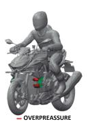
Due to its angles and frontal surface, it creates an overpressure on the top of the spoiler.
