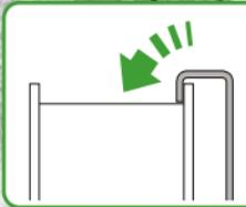
Ensure radiator guard securely hooks over the top lip of the radiator
