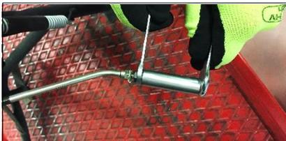
**ENG** Insert the cable with the adjuster body inside the protection, tighten with a wrench 8 mm for the adjuster body and with a wrench 13 mm for the protection.
