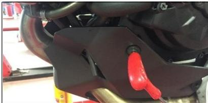
**ENG** Remove the skid plate unscrewing the screws on the right and left side
