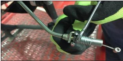
**ENG** Insert the cable in the seat and screw the adjuster body, tighten with a wrench 8 mm for the adjuster body and with a wrench 10 mm for the nut on the cable.
