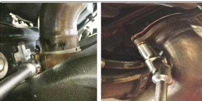
**ENG** Tighten the exhaust system starting with the screw of the silencer support bracket, the small metal clamp, till the nuts of the head pipe.
