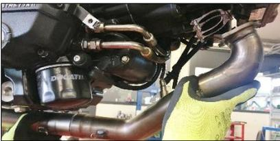
**ENG** Start to positioning the collector by placing it into the horizontal head pipe
