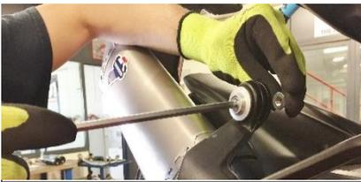
**ENG** Screw the silencer support bracket to the frame using the original screw, washer and nut, placing the washer between the frame and the bracket and the nut behind the bracket.
