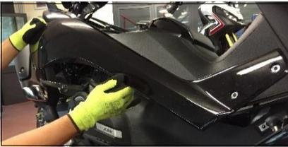
**ENG** Open the saddle, unscrew and remove plastic cover on right side
